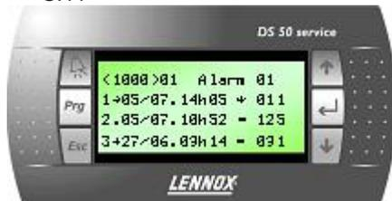
The history can store the last 32 alarms occurring on the unit. Each alarm is memorised at the date and time of occurrence of the fault. An active alarm is signified by the symbol '\*'. An acknowledged alarm is signified by the symbol '='. Each alarm is signified by a 3 digit code (see ERROR CODES)
