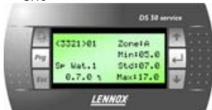
If the period of operation is displayed on the first line, the parameter in question can be set to a different value for each for each period (Z.A, Z.B, Z.C, Uno and BMS). To display and change the values of other periods, press the 'Prg' button. Pressing the 'Prg' button confirms the change in the same way as button ←.
