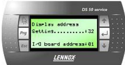
Access the configuration mode by pressing the buttons  $\uparrow$   $\downarrow$   $\leftarrow$ , for at least 5 seconds until the Sds.1 screen appears:
