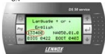
In the case of a specific program for one job (NSR), this is identified by the display of a factory number to the left of the S.4 program version.
