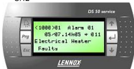
Pressing the 'Alarm' key for more than 10 seconds resets the history of the 32 alarms to zero.
