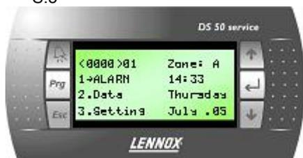
The four digits in brackets indicate the number of the current menu. The two digits beside the brackets indicate the pLan number of the selected card. The display on the right indicates the period of operation and the current time conditions.
