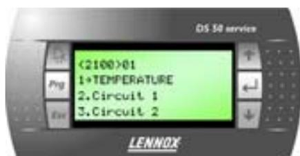
Press "Esc" at any time sends to return to the previous level of the menu tree. In the example shown above, "Esc" must be pressed 3 times to return to the main menu (0000)
