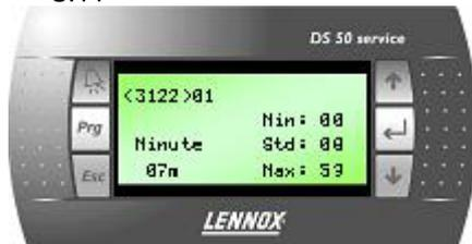
Screen S.14 is used to change a set point (e.g. Minutes p.3122). The maximum and minimum thresholds for the parameter are displayed on the right of the screen, as well as the predefined default value. With button ↑ or ↓ set the desired value and confirm with button ←.
