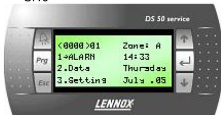
In the event of an alarm on the unit, the 'Alarm' button is illuminated in red. In the event of a filtration fault, the 'Prg' button is illuminated in yellow.
