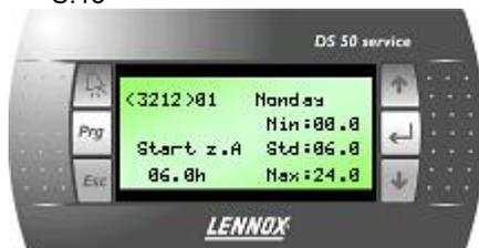
If the day of the week is displayed on the first line, the parameter in question can be set to a different value for each day of the week. To display and change the values of other days, press the 'Prg' button. Pressing the 'Prg' button confirms the change in the same way as button ←.
