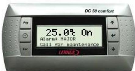
In the event of activation of a fault on the unit, screen Sdc.8 is displayed.
