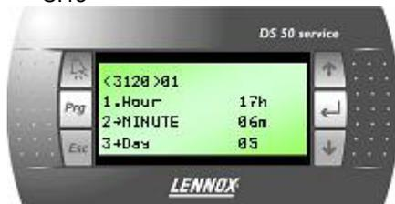
To change a parameter on a set point; Select the 'SET POINTS' line from the main menu, then navigate to the sub-menus until the desired set point is displayed (e.g. 3120). Position the cursor over the line desired (e.g. 2.) then confirm with button ←.
