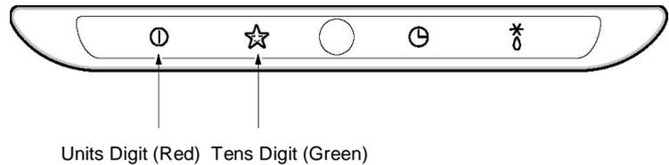
The “Units” digit of the fault code is shown by the power led which has the following symbol by it This is usually Red, but on a few models it is Green.
