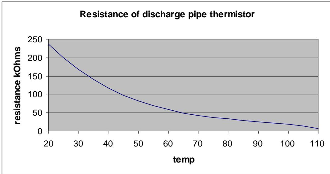
Alternatively the sensor can be tested while still connected to the PCB measure the DC voltage across the resistor and check it against the graph below.
