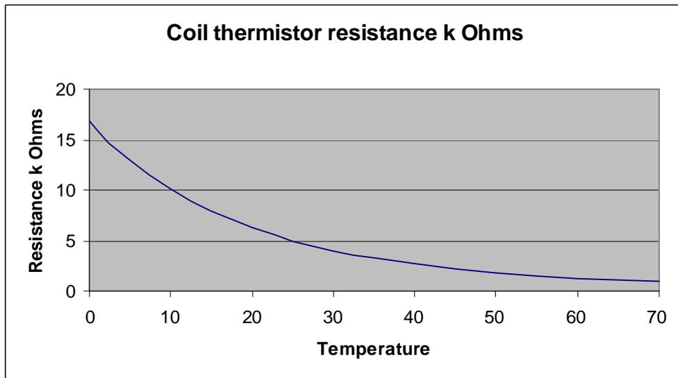
Alternatively the sensor can be tested while still connected to the PCB measure the DC voltage across the resistor and check it against the graph below.
